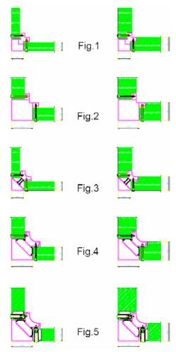
New 60 mm thick cold bridge free profile (see construction details shown in Fig. 5), made separating the metal sheets and placing an extruded plastic layer of more than 40 mm in thickness inbetween, is able to achieve with special structural features and innovative heat insulation materials an overall casing U-value of T1 in accordance with the provisions of UNI EN 1886.
